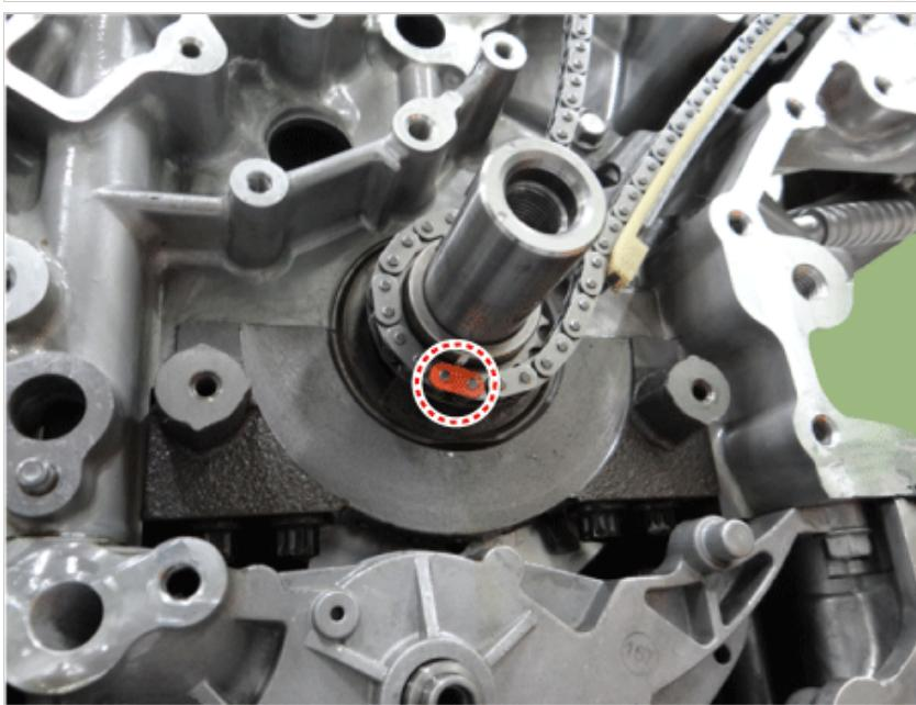
6. Install the LH timing chain tensioner arm (A).
